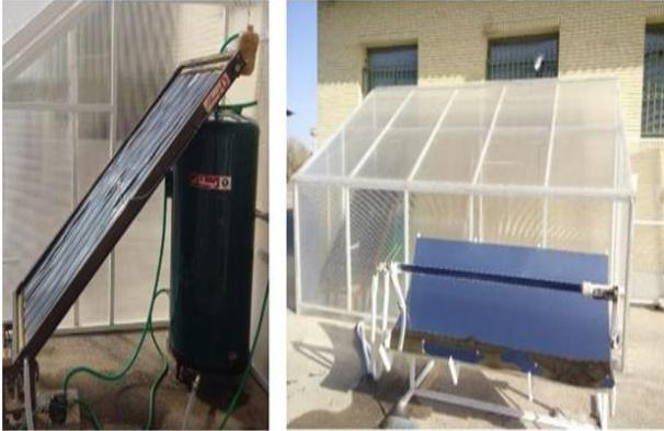
**Fig. 2.** A photograph of the designed solar heating system and the greenhouse; a) The modified FPC and the tank inside the greenhouse and b) the PTC assembly
