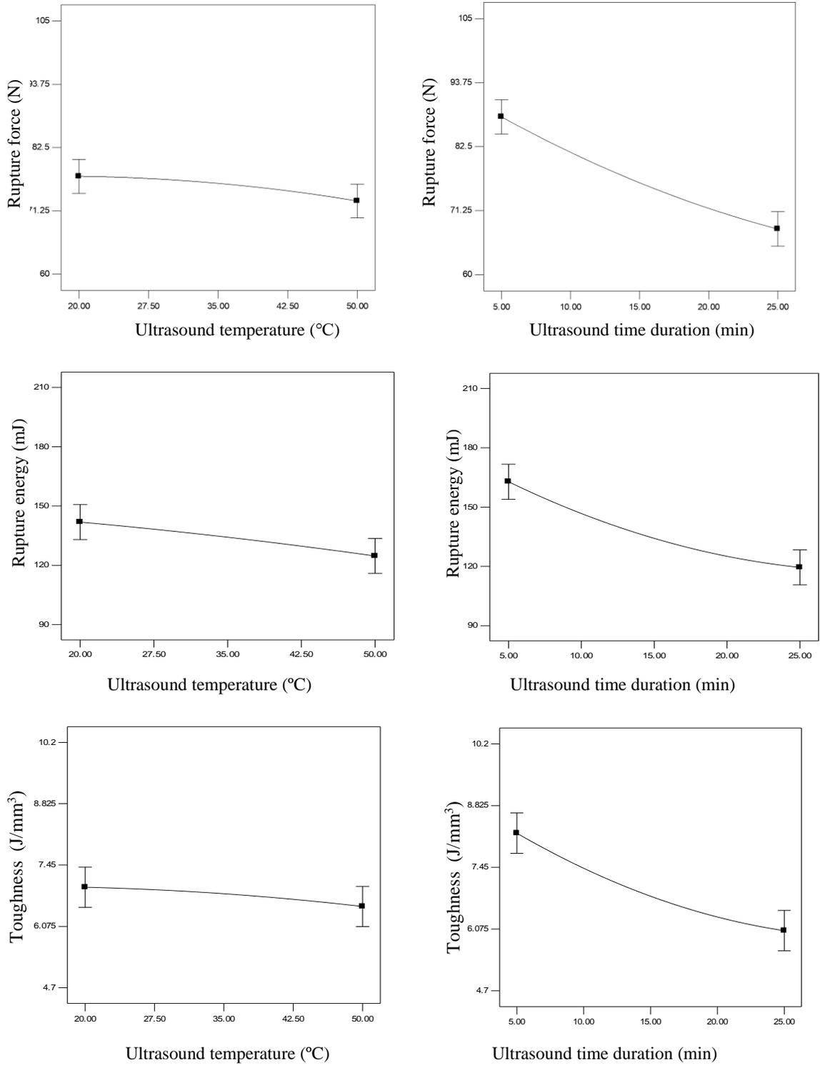
**Figure 3.** Mean values of rupture force, required energy, and toughness compressed at different ultrasound time duration and different ultrasound bath temperature.
