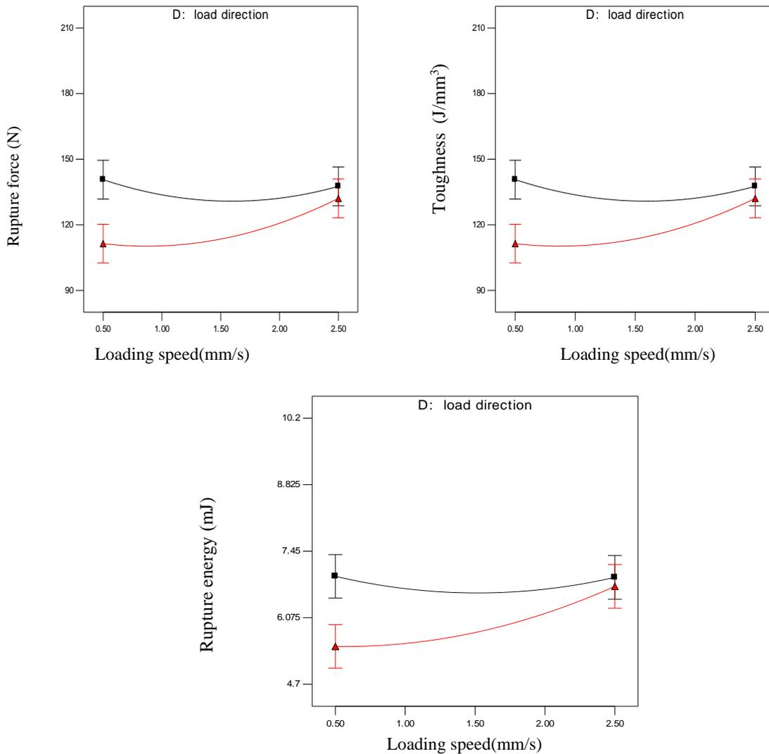
**Figure 5.** Interaction effect of loading speed and direction on mechanical properties of walnut (■ Longitudinal loading ▲ Latitudinal loading)
