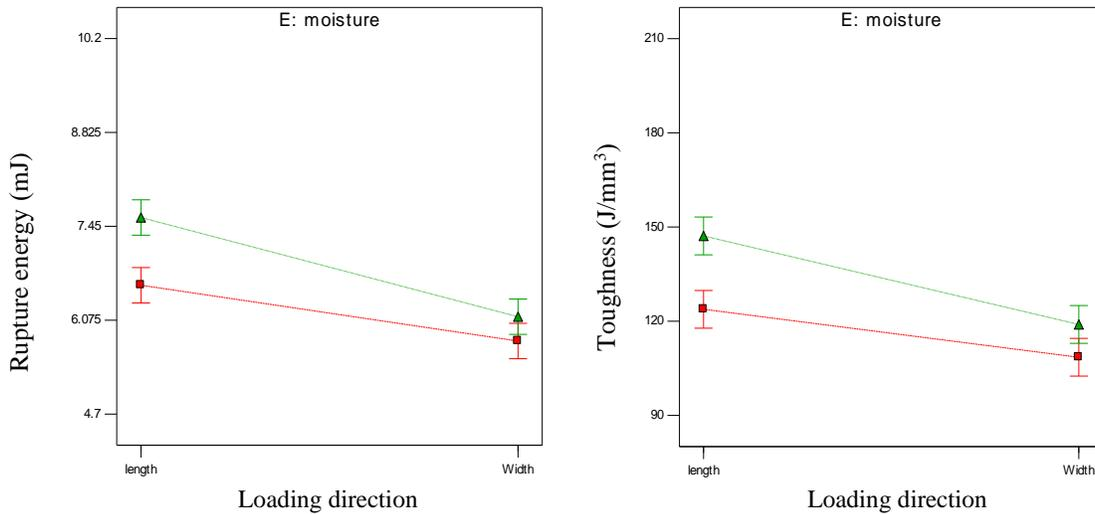
**Figure 4.** Interaction effect of loading direction and moisture content on rupture energy and toughness (■ Wet walnut ▲ Dried walnut)
