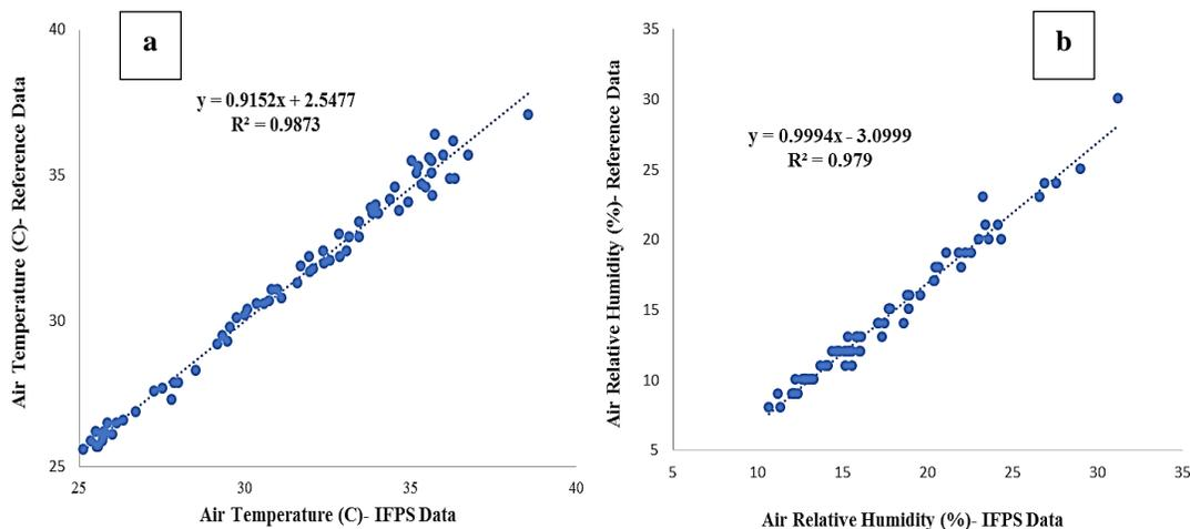
**Figure 3.** Comparing the air temperature (a) and air relative humidity (b) recorded by the IFFS with the data recorded by the reference sensor
