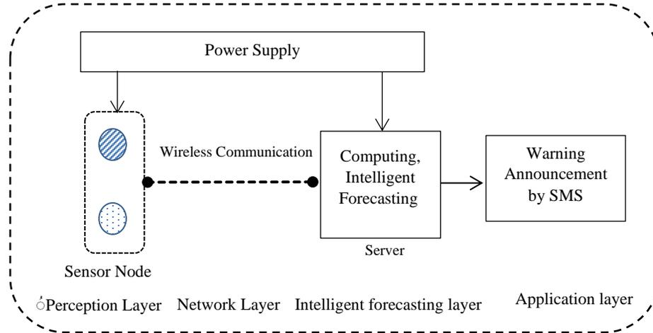
**Figure 2.** The IoT-based block diagram of the IFFS
