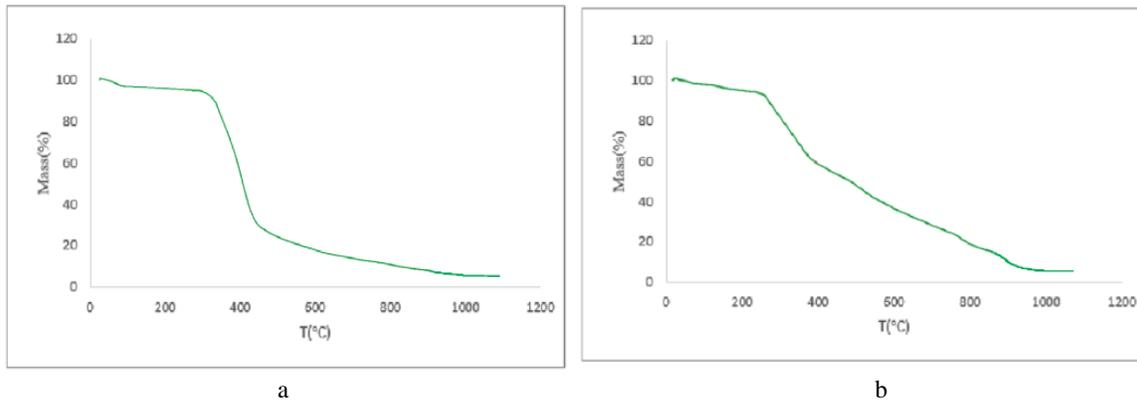
**Figure 1.** Thermal weighing of pistachio stem (a) and pistachio leaf (b)
