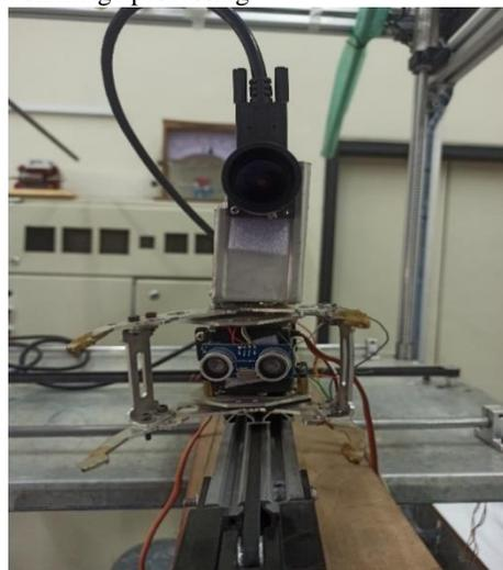
**Figure 4.** camera and depth sensor position related to gripper
