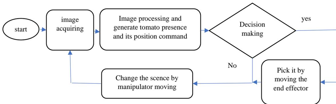
**Figure 3.** tomato detection algorithm based on image processing
